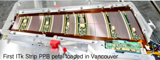
First ITk Strip PPB petal loaded in Vancouver
