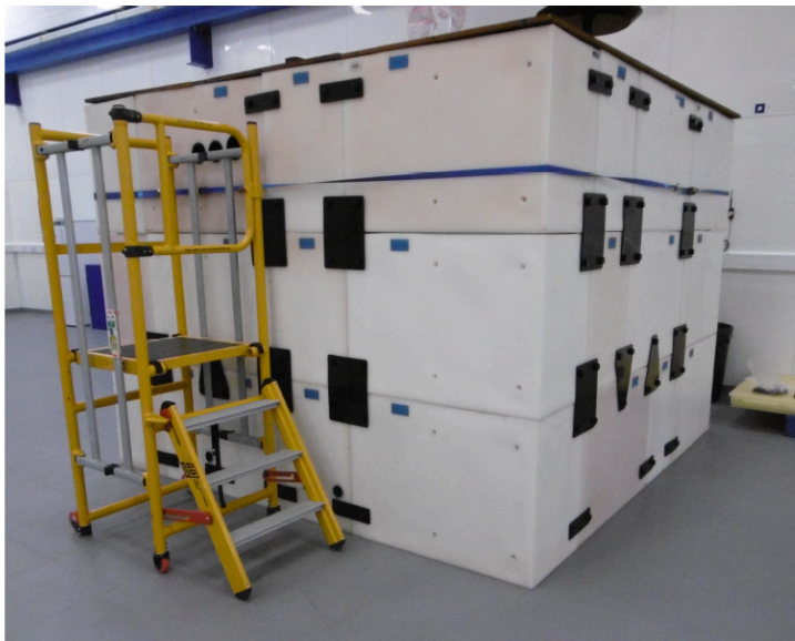
FIG. 25. DRIFT-II d interlocking acrylic block shielding surrounding the detector and containing water, located at Boulby underground laboratory.
