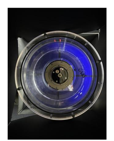
3D printed flange holding up PMT with rubber Oring
